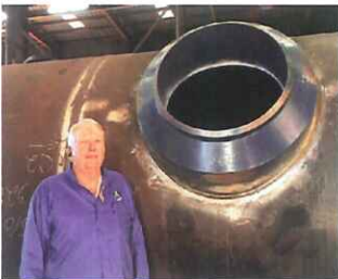
Gulfex Holdings LLC President Aubrey W. Davis stands beside a vessel boot forging manufactured by Forged Components Inc. (FCI) and installed in a Gulfex Holdings LLC vessel in fabrication.
