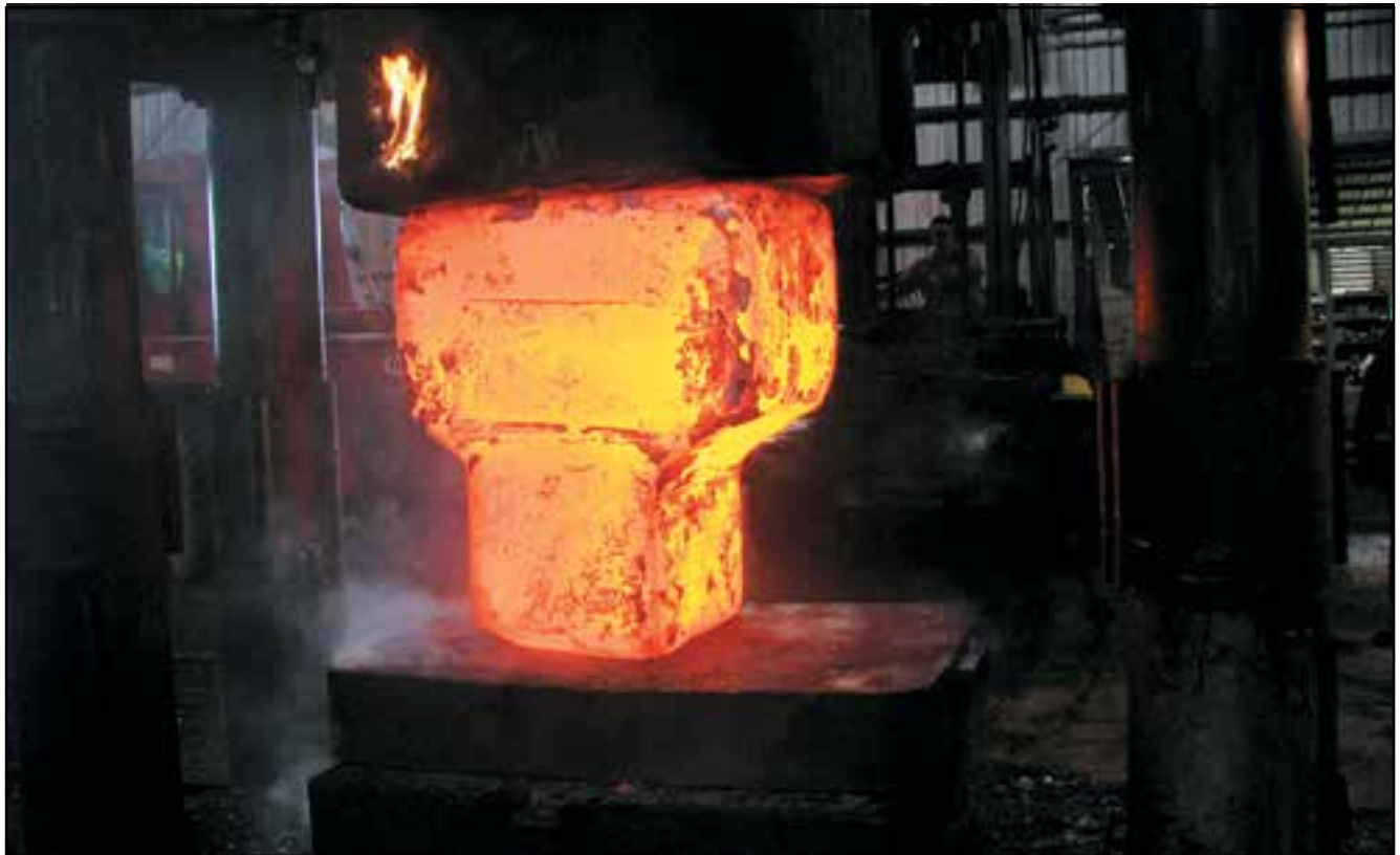
19,000 Lb Pigable Y Block Forging
