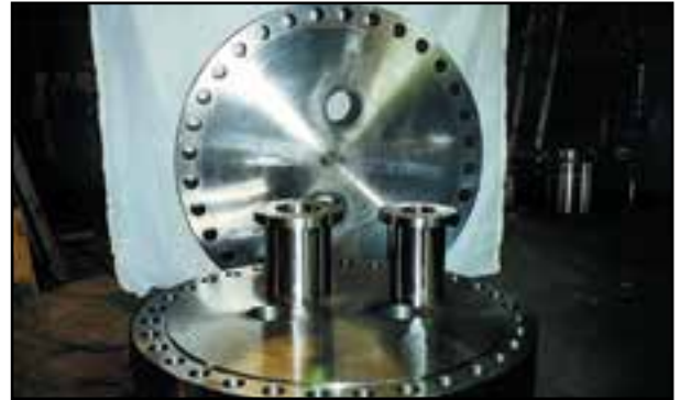
Blind Flanges and "LWN" Connections
