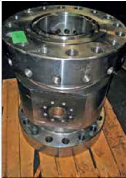
Tubing Head 13 5/8" 5M x 11" 10M with 1 13/16" 10M Outlets
