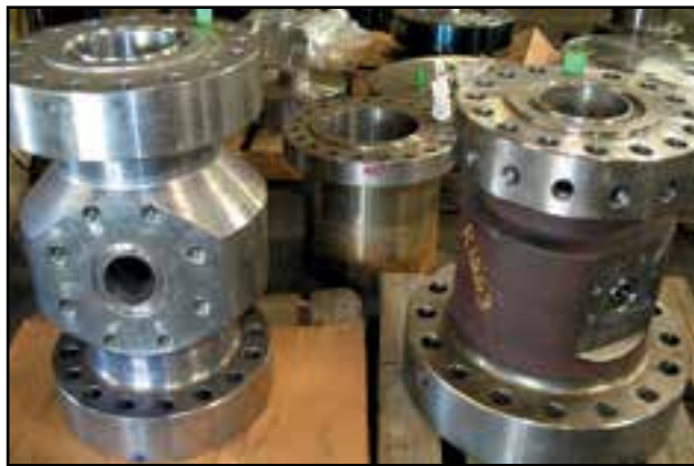
15M and 10M Spool with Studded Outlets
