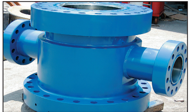
20 3/4" 3M x 16 3/4" 5M Spool with 9" 5M EFO's
