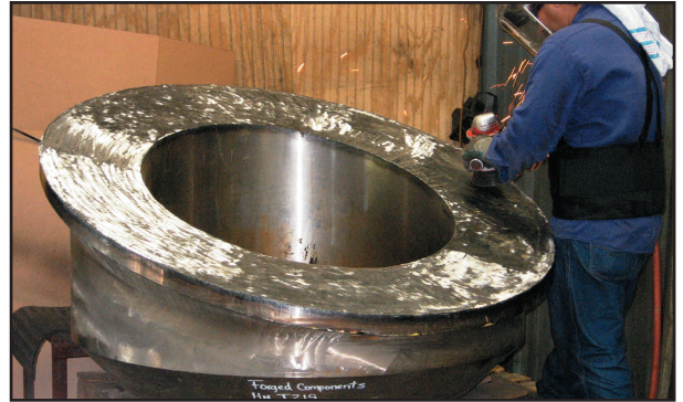
36" F11 Hillside Q-Lip Stubs for Coker Vessels
