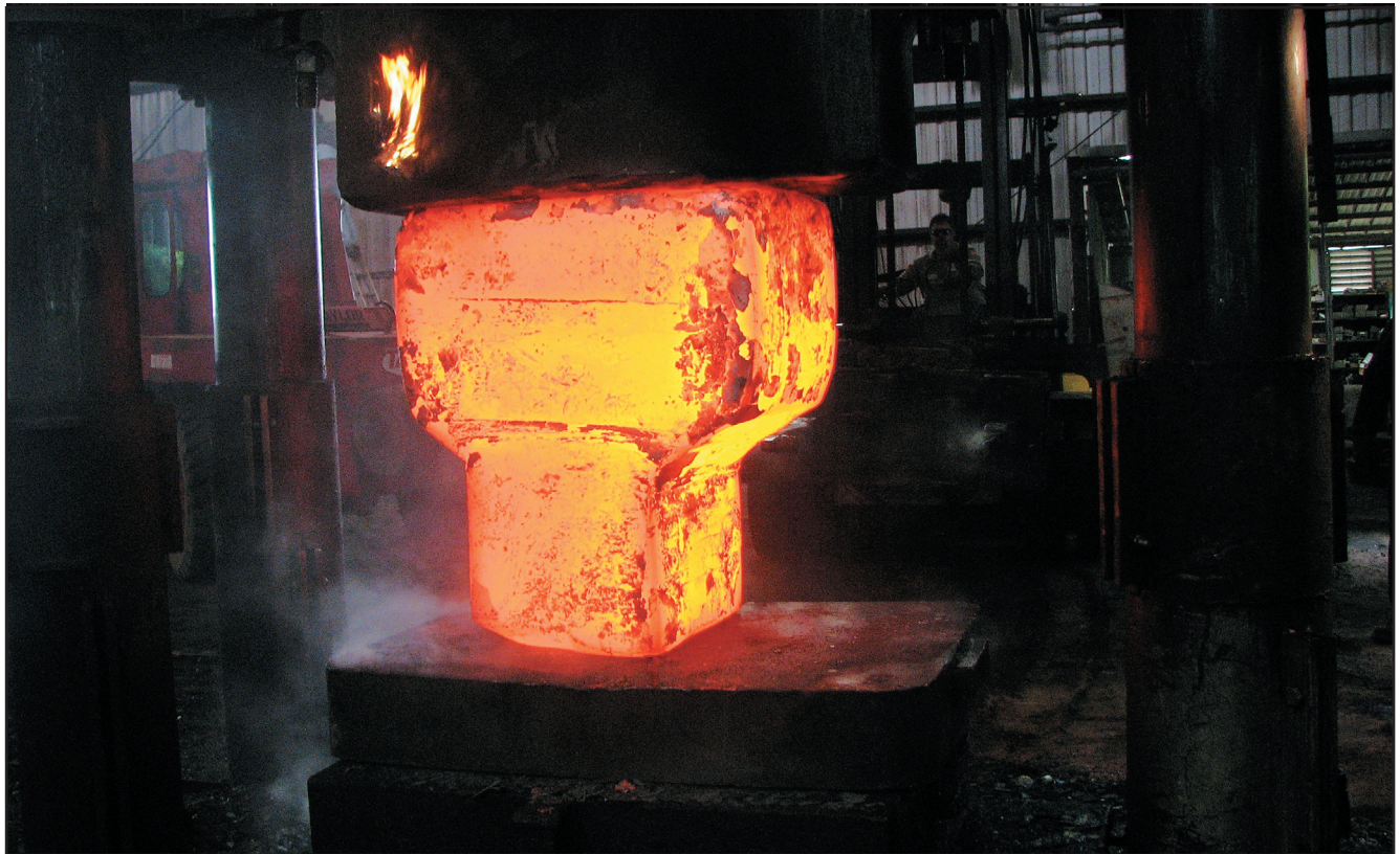
19,000 Lb Pigable Y Block Forging
