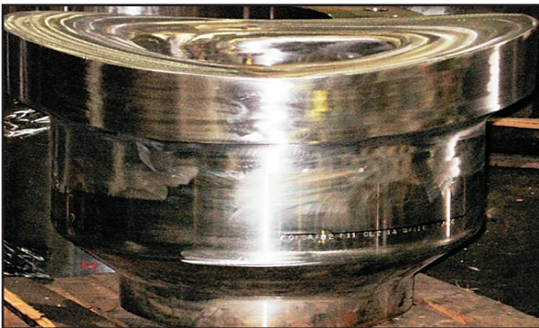
F11 Heavy Wall Q-Lip Stub
