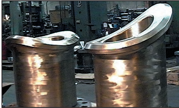
HB Necks Q-Lip Style for Radial Attachments and Cylindrical Hillside Complete with Bevels
