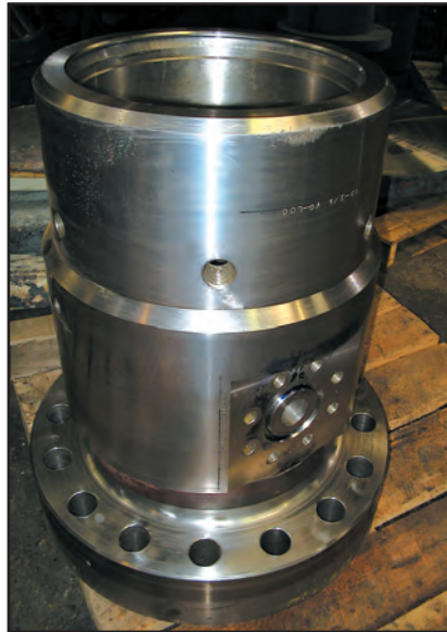
11" 10M Lower Slip Loc Housing with FPO's
